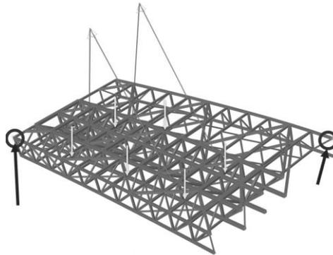
Figure 3. Position of fictitious lateral restraint
