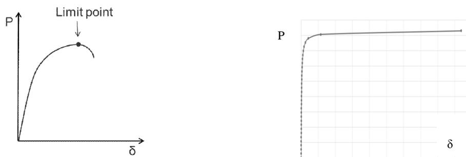
Figure 5. Buckling limit reached by unloading (Left). Buckling limit reached by convergence criterion (Right)
