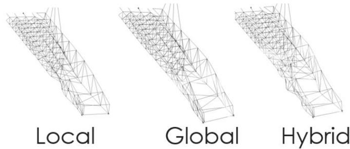
Figure 4. Buckling Modes of a Structure
