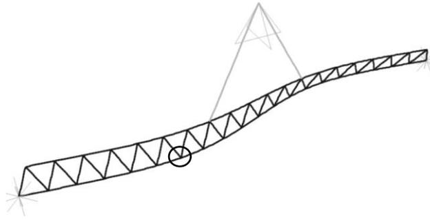
Figure 7. Shape of the 3<sup>rd</sup> Buckling Eigenmode. Circle marks the location with maximum displacement.
