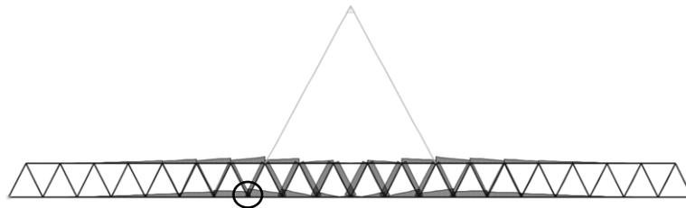
Figure 8. Buckling Modes of a Structure. Circle marks the location with maximum stress.
